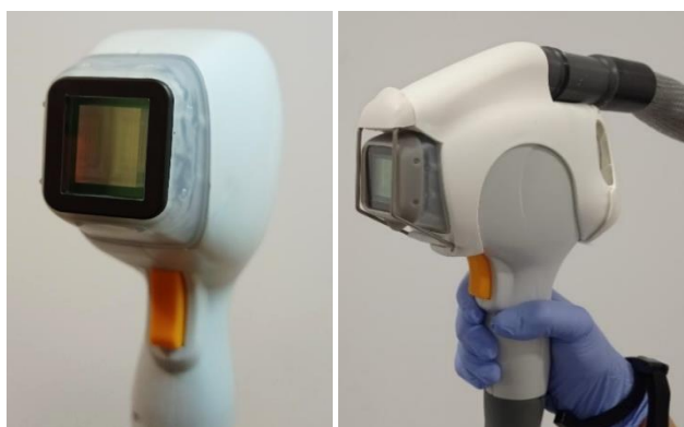
Figure 1. 4,800 W, 810 nm, 20x15 mm diode laser applicator (left). Air-cooling accessory mounted on the 20x15 applicator (right).
